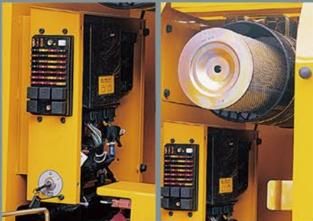
Centralized Electric Control Box and Easy Change Air Cleaner Assembly Electric control box and Air cleaner are centralized in one or the same compartment for easy service.
