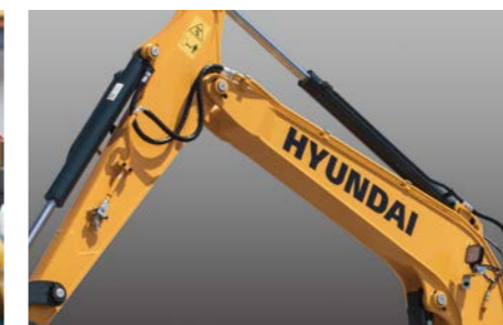
Standard breaker piping
