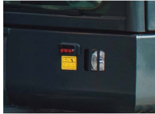
Centralized grease system
