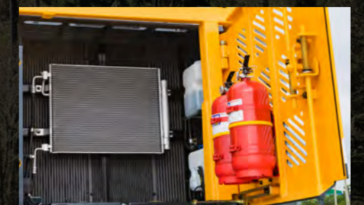
Fire extinguishers in left side cover and inside cabin
