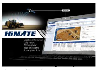
Hi-mate, Hyundai's proprietary remote management system, provides operators and dealer service personnel access to vital service and diagnostic information on the machine from any computer with internet access. Users can pinpoint machine location using digital mapping and set machine work boundaries, reducing the need for multiple service calls. Hi-mate saves time and money for the owner and dealer by promoting preventative maintenance and reducing machine downtime.
