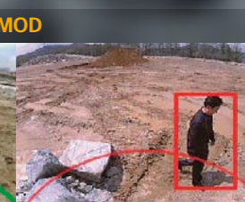
A red warning sign is displayed when people move in within a 3-meters radius.
