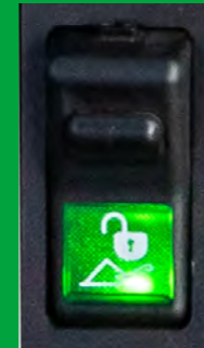
Safety Switch (loader)
