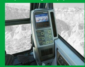
Instrument Panel is installed in front of RH console box. It is easy to check all critical systems with easy-
