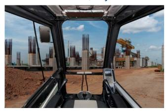
The cab is roomy and ergonomically designed with low noise level and good visibility. A full view front window and large rear and side windows provide excellent visibility in all directions.
