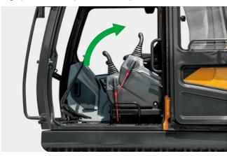
New joystick grips for precise control have been equipped with double switches.
