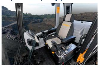
All the controls are designed and positioned according to the latest ergonomic research. Reinforced pillars have also been added for greater cab rigidity.
