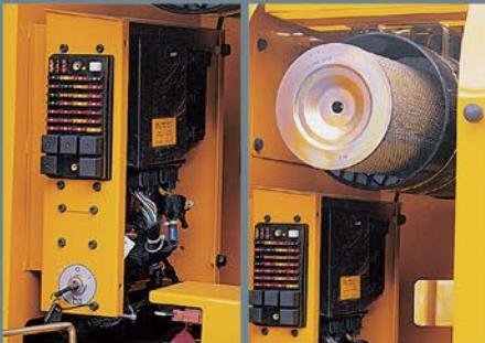
Centralized Electric Control Box and Easy to Change Air Cleaner Assembly Electric control box and Air cleaner are centralized in one or the same compartment for easy service.
