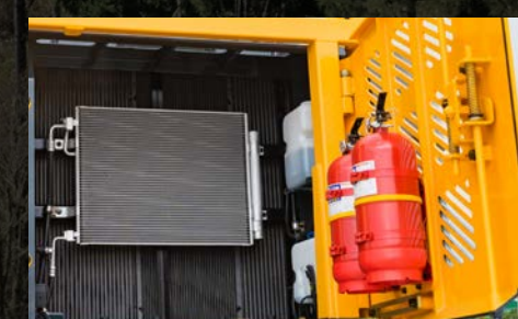
Fire extinguishers in left side cover and inside cabin
