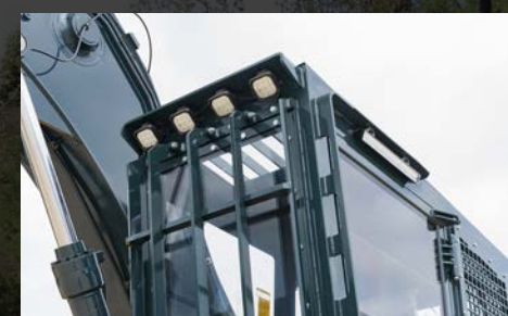
LED lamps on front, left and rear side of cabin
