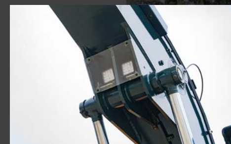
LED boom lamps and lamp cover
