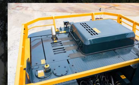
Heavy duty rear guarding rail and full protection rail
