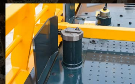
Fuel and hydraulic oil inlet guards
