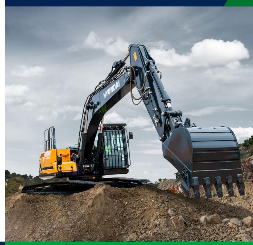
Gross Power 160 HP (119 kW) at 2,200 rpm **Net Power** 157 HP (117 kW) at 2,200 rpm Bucket Capacity 0.92 ~ 1.34m<sup>3</sup> **Operating Weight** 21,970 kg / (48,440 lb)
