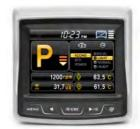
Self diagnostics, color rear-view camera maintenance check lists and start-up machine security, were integrated into the monitor to make the machine more versatile and the operator more productive. The new monitor display unit is mounted on an adjustable swivel mount to reduce glare and position according to operator preference.
