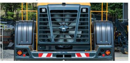
The remote mounted, hydraulically powered cooling fan regulates fan speed according to working temperatures for coolant, intake air, transmission oil and hydraulic oil. This new fan design contributes to reduced fuel consumption and machine noise. The fan is designed to auto reverse periodically or manually reverse to keep debris from accumulating on the coolers. (Manual mode: Reverse only when switch is pressed)
