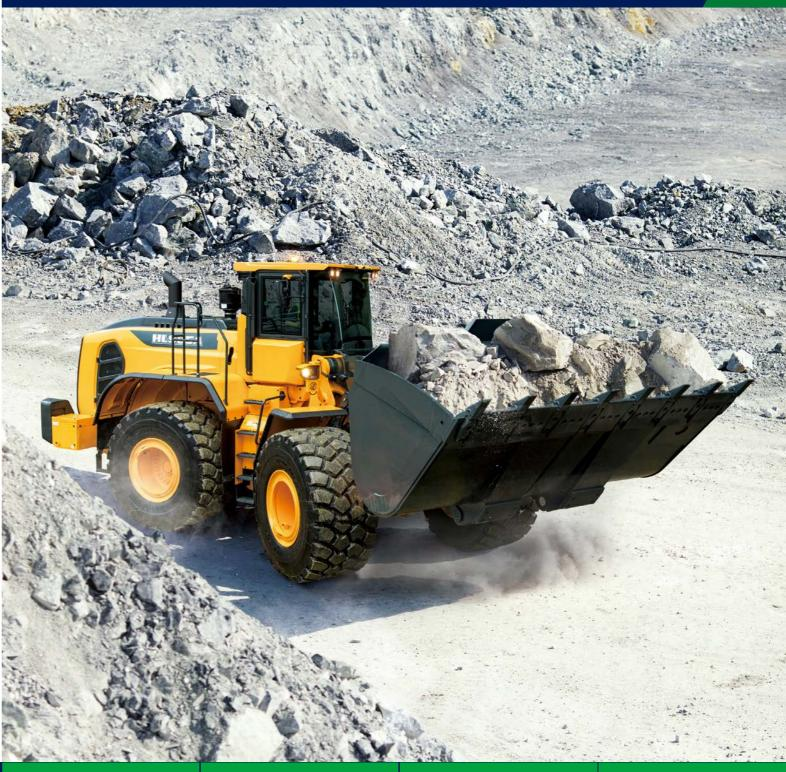
Gross Power 430 HP (321 kW) 2,100 rpm **Net Power** 420 HP (313 kW) 2,100 rpm Bucket Capacity 6.5 ~ 7.0 m<sup>3</sup> Operating Weight 33,800kg / 74,520 lb
