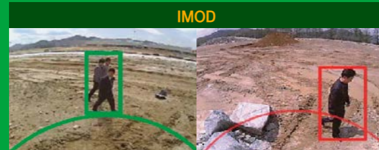
A green warning sign is displayed when people move in within a 5-meters radius.
