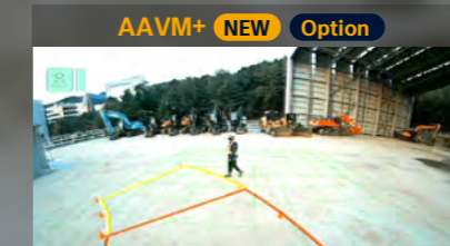
It offers reverse guidelines and a feature that alerts you only to objects detected in the reversing path.
