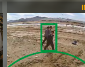
A green warning sign is displayed when people move in within a 5-meters radius.
