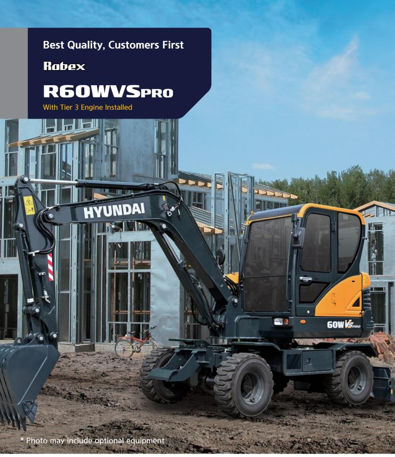
Rated Power: 42.5kW / 2,400rpm | Operating Weight: 5,750kg | Default bucket capacity: 0.21m³ (SAE heaped)
