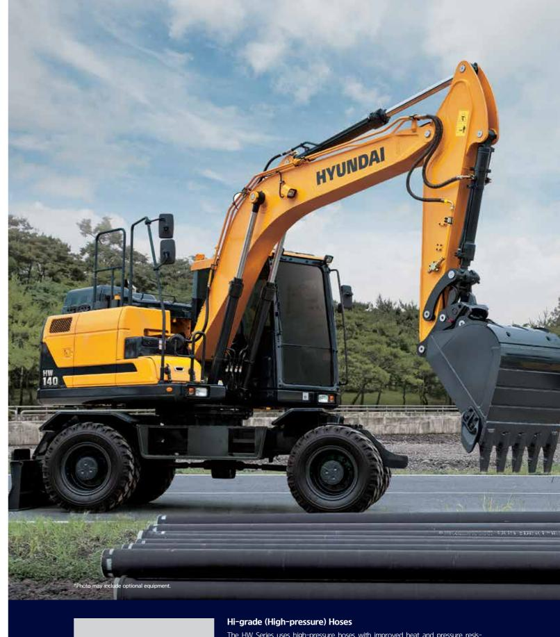
The HW Series uses high-pressure hoses with improved heat and pressure resistance, greatly increasing the durability of the equipment.
