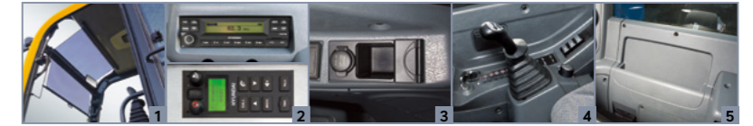
Sun screen Radio & USB player with remote control and blue tooth hands free Hands-free cell phone Joystick Storage compartment
