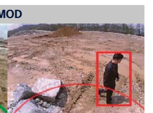
A red warning sign is displayed when people move in within a 3-meters radius
