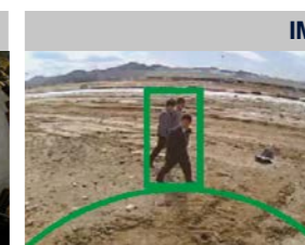
A green warning sign is displayed when people move in within a 5-meters radius.
