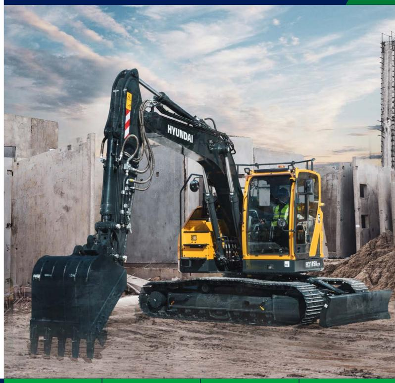
Gross Power 100 kW (134 HP) at 2,200 rpm **Net Power** 98 kW (131 HP) at 2,200 rpm Bucket Capacity 0.50 ~ 0.77 m<sup>3</sup> Operating Weight 15,430 kg / 34,020 lb
