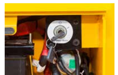
Battery master switch
