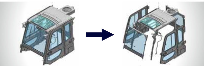
Bolt on type cabin The bolt on type cabin consists of front side, door front, door rear, and rear side. It is easy to assemble by bolt and mount parts. Also, cabin can be selected by module or parts and air conditioner and heater are separately available for driver's convenience.
