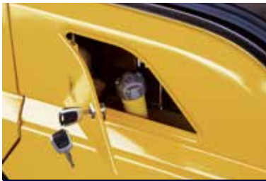
Fuel cover with key The key on the fuel inlet door prevents people from stealing fuel.
