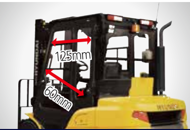
Wide cabin (OPT) A wide cabin can be selected (60 mm wide and 125 mm long) for wider indoor space.
