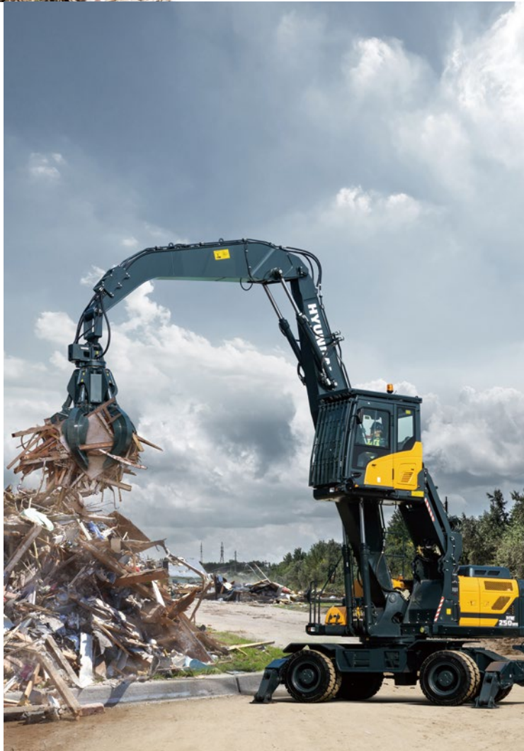
Streamlined electric excavator capable of performing various tasks such as buckets, waste handling, and hoppers with the powerful output of the electric motor mounted on the equipment
