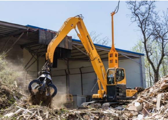
Streamlined electric excavator capable of performing various tasks such as buckets, waste handling, and hoppers with the powerful output of the electric motor mounted on the equipment
